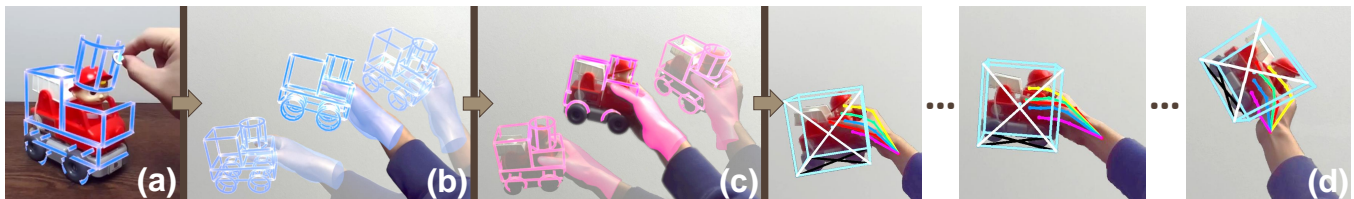
Figure 1: Overview of the ARnnotate workflow. (a) A user creates a bounding contour as the virtual representation of a target physical object in AR. (b) The user manipulates the bounding contour with a preferred gesture, while ARnnotate keeps recording the 3D poses of both the bounding contour and hand obtained by a hand-tracking-capable AR-HMD as the dataset labels. (c) ARnnotate replays the record as an interaction clip in AR. The user grabs the physical object using the same gesture and manipulates it while ensuring both the hand and object are accurately aligned with the counterparts of the interaction clip . ARnnotate captures the user's first-person view as the dataset images and temporally pairs them with the corresponding labels via back-end processing. (d) The custom dataset created by ARnnotate.
