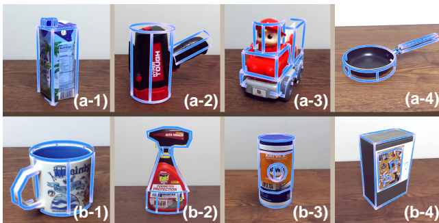
Figure 3: Example bounding contours created by ARnnotate. (a-1 to a-4) Bounding contours created by the primitive creation method. (b-1 to b-4) Bounding contours created by both the primitive creation and free-sketch creation methods.
