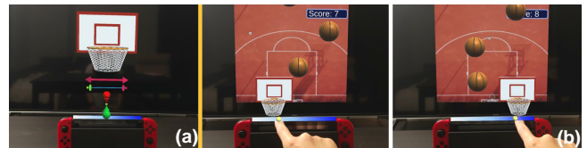
Figure 7: Gaming Controller: (a) The 'upper' continuous edge is connected to the virtual basket's 'horizon translation' behavior. (b) Then the user can slide his finger on the edge to let the basket catch falling basketballs.
